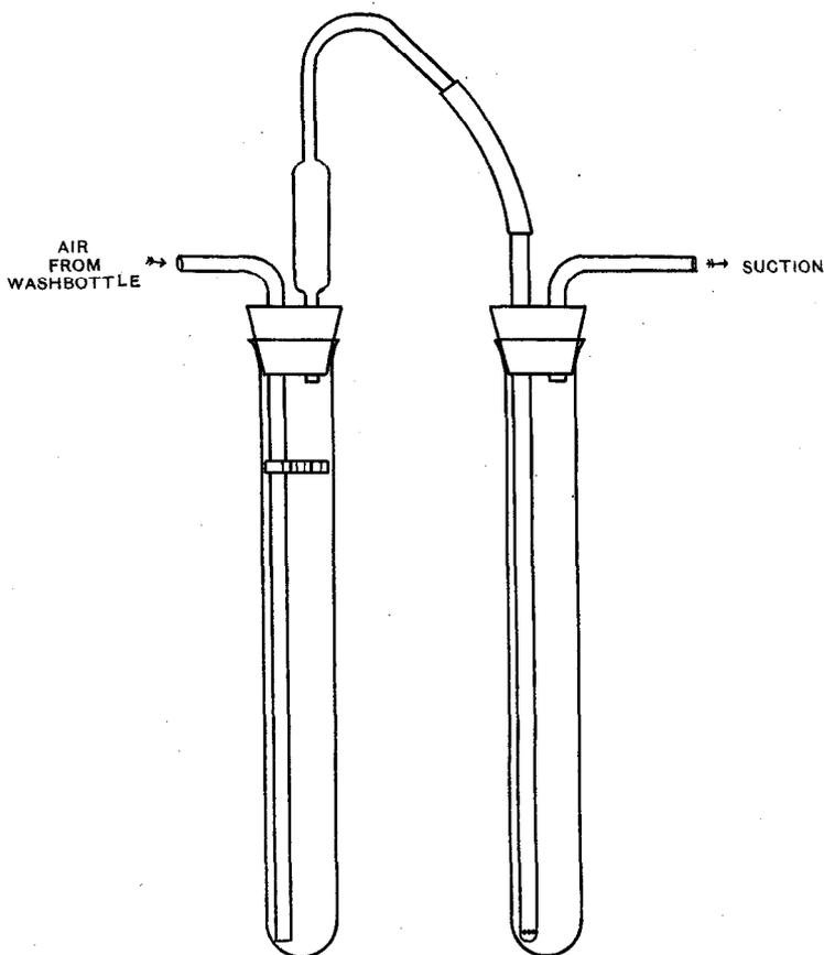
FIG. 2. APPARATUS FOR USE WITH SUCTION.
